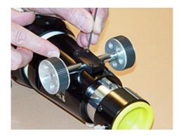
**1.b.** Using the 5/64 Allen wrench remove the (4) Button Head Cap Screws.
