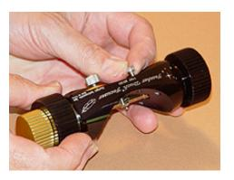
**2.b**. Insert the (4) Socket Head Cap Screws into the Housing as shown.
