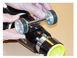
**1.d.** Remove the pinion assembly.
