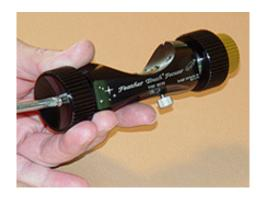
**2.a.** Remove the Feather Touch TVRF from the shipping box. Insert the coarse focuser knob on the pinion and fasten it with the Phillips screw that is supplied. Hold the knob firmly while tightening the screw. Use a good Phillips screw driver so that the knob can be properly tightened. Be careful not to slip.
