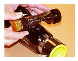
2.c. Place the Feather Touch Micro Pinion Assembly onto the TV focuser housing and move it back and forth slightly until you can feel the pinion and the screws nest into position.
