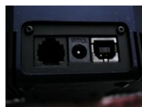
Electrical panel on bottom of QSI camera
