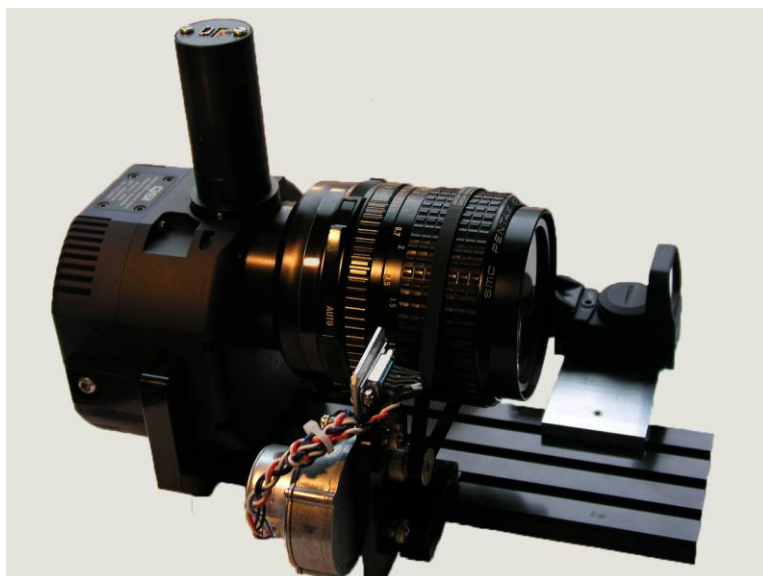
QSI583WSG with Lodestar guide camera mounted on QSI Dovetail Camera Mount, with Hurst focus motor, QSI 67 lens adapter, Pentax 67 55mm f/4 lens, prototype red dot finder plate, and red dot finder.
