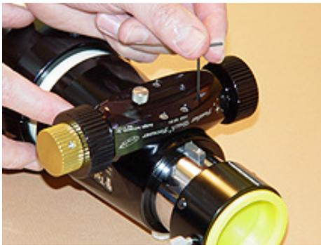
**2.e.** Insert the 1/16 Allen wrench into the adjustment hole and tighten the leveling screws on the front side until you can feel that contact is made between the leveling screw and the focuser housing. Do this for both sides. Then work on the back screws repeating the same steps.
