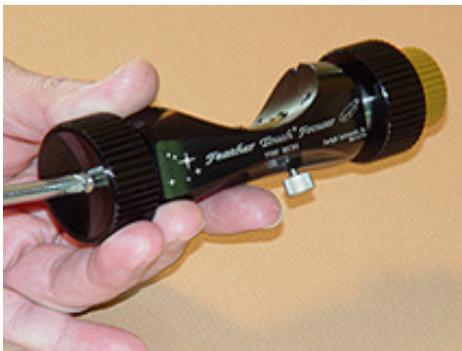
2.a. Remove the Feather Touch TVRF from the shipping box. Insert the coarse focuser knob on the pinion and fasten it with the Phillips screw that is supplied. Hold the knob firmly while tightening the screw. Use a good Phillips screw driver so that the knob can be properly tightened. Be careful not to slip.
