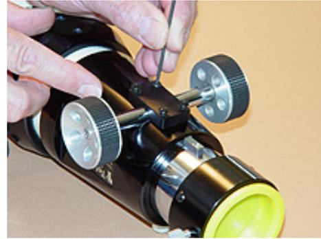
1.b. Using the 5/64 Allen wrench remove the (4) Button Head Cap Screws.
