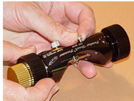
2.b. Insert the (4) Socket Head Cap Screws into the Housing as shown.
