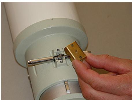
**1.f.** Remove the pinion saddle.
