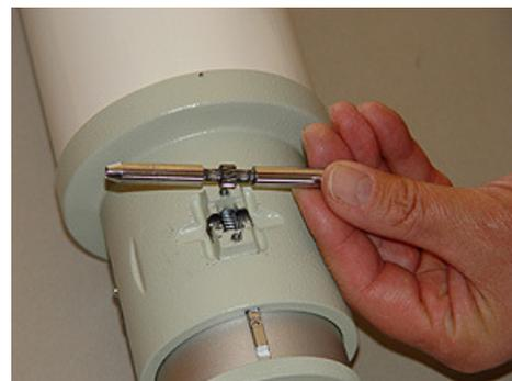
**1.g.** Remove the pinion from the focuser housing and place it on a clean piece of paper or paper towel.
