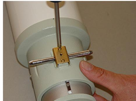
**1.e.** Remove the two Phillips screws that holds the pinion saddle in place.
