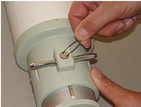
**1.d.** Remove the pinion cover nut using the supplied spanner spring as shown. Turn the nut counter clockwise to loosen.
