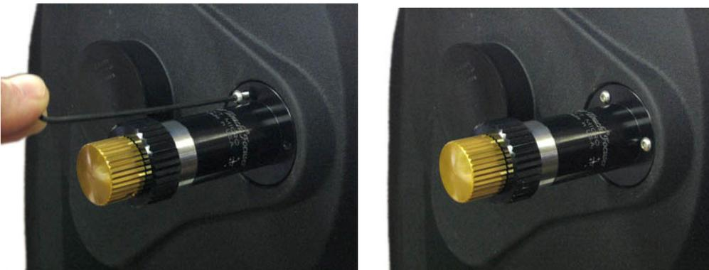
Use the three provided hex-head screws and wrench to attach the SCT MicroFocuser to the telescope. You are now ready to head out under the stars! Use the black knob for coarse focus and the brass knob for fine focus (10:1 ratio). Note that the telescope will likely be pretty far out of focus, so you may need to turn the focus knob quite a few times to reach focus.
