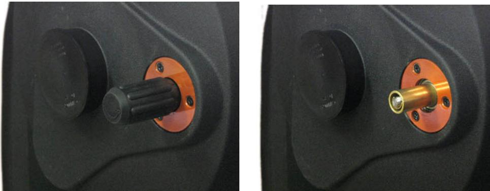
Begin by removing the black rubber focus knob from the scope. This knob simply pulls off the brass focus cylinder.
