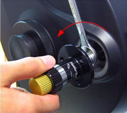
Thread the MicroFocuser into the brass stop. Hold the stop with a wrench and the black focus knob with the other hand to tighten the stop. *This stop MUST be tight to secure the MicroFocuser to the focus shaft.*
