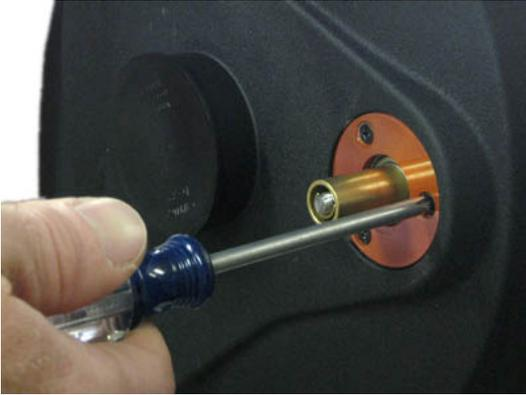
There are 3 small Phillips-head screws which hold the orange focus assembly cover in place. Remove these screws and take off the flat cover plate, exposing the inside of the focus assembly.
