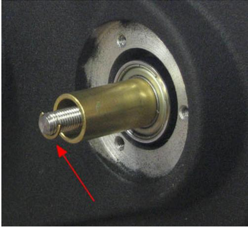
The C-clip at the end of the focus shaft must be removed to install the SCT Micro-Focuser. The clip should be removable by hand, but you may use needle-nose pliers or a similar tool if necessary. Be careful not to scar the threads of the focus shaft as the SCT MicroFocuser must be threaded on in a later step. If your telescope has a screw and washer, simply remove these with a screwdriver. Keep these parts handy; they will be reinstalled later.
