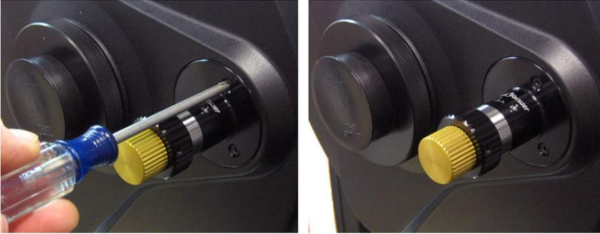
Use the three original screws to attach the SCT MicroFocuser to the telescope. You are now ready to head out under the stars! Use the black knob for coarse focus and the brass knob for fine focus (10:1 ratio). Note that the telescope will likely be pretty far out of focus, so you may need to turn the focus knob quite a few times to reach focus.
