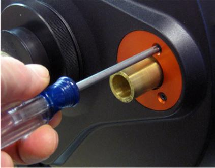
There are 3 small Phillips-head screws which hold the orange focus assembly cover in place. Remove these screws and take off the flat cover plate, exposing the inside of the focus assembly. These screws will later be used to attach the MicroFocuser.
